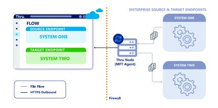
When a flow's source and target locations are on the same network and the endpoints are served by the same Thru Node, the file remains on the network and is not exposed to the internet. The file is moved from the source to target location over the network's file system or file transfer protocols such as NFS, SMB, SFTP, FTPS or HTTPS. The metadata associated with the file transfer is transmitted via an outbound connection to Thru cloud over HTTPS and is recorded in Thru Audit.
